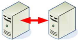
The design will be deployed on two physical servers, using a Virtual Machine environment with four virtual servers per machine. Each server will host a load balancer, a web server, a file server, and a database.
